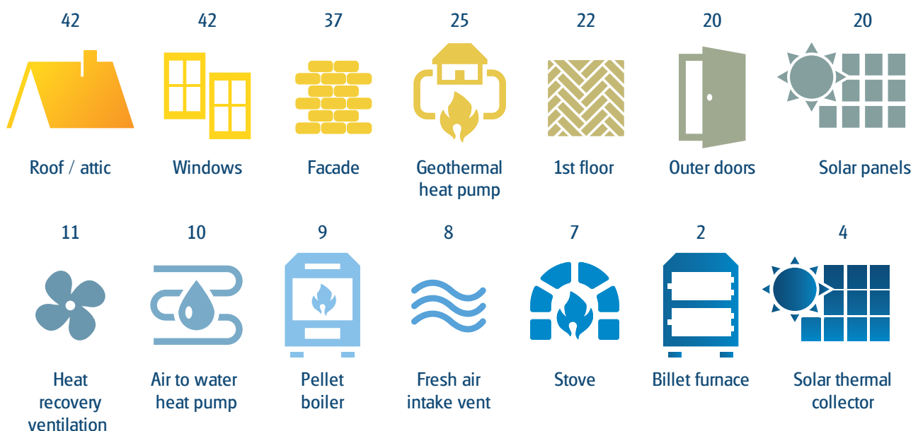
Figure 11. Works performed with the grant for increasing the energy-efficiency of small residential building:
